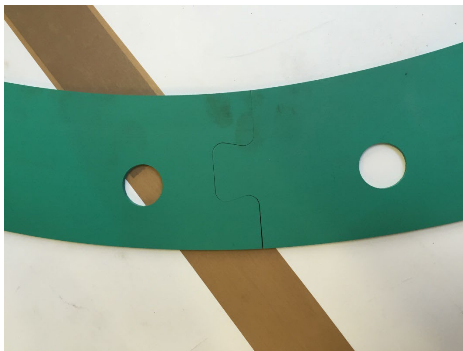
Figure 3 OK for Post Bake discolouration
