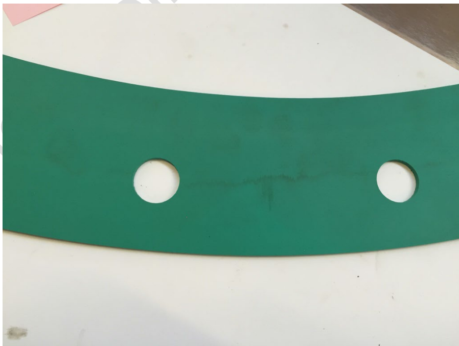
Figure 2 OK for discolouration and flow marks
