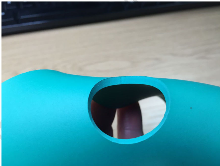
Figure 6 OK for Hole Stop/Start Point of Cutting Machine
