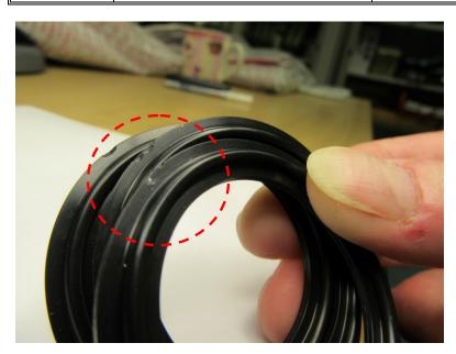
Chipped OD from CRYO trimming, this is not acceptable.
