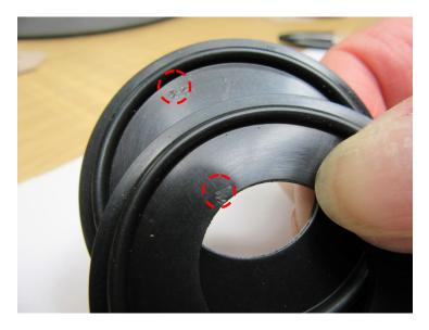
Poor Surface finish on sealing area, not acceptable.
