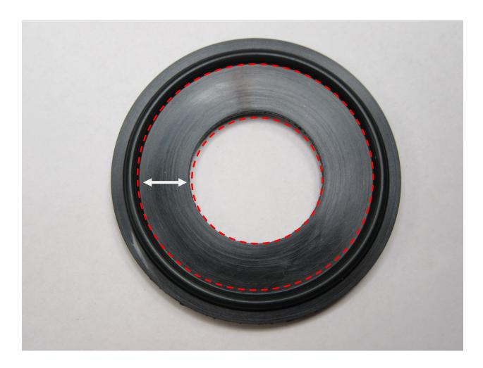
Area indicated between dotted lines is the critical sealing surface, including inside diameter. Other areas are non-critical. They are to be visually inspected using good lighting, 2 X magnification is not required unless to verify defect type.
