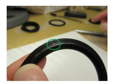
Damaged tool mark on non-critical sealing area, this is acceptable.
