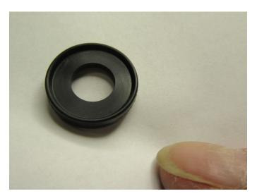
Good surface finish on Sealing area and no excess flash on ID.
