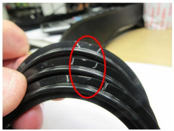
Breaking away on noncritical area, excessive depth, unacceptable.
