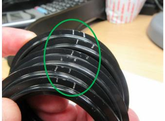
Breaking away on noncritical area, minor depth, acceptable.
