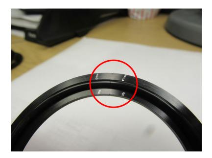
Poor flow of material at moulding stage, not completed in cavity, appears on both sides of seal, this is not acceptable.
