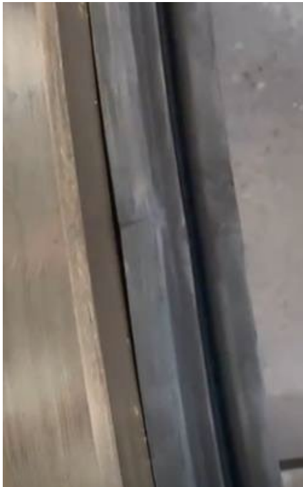
Image 8 Unacceptable join quality, seal fitted in Rothe Erde Housing
