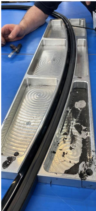
Image 2: TBMS Seal fitted into housing JWC-PD-210070
