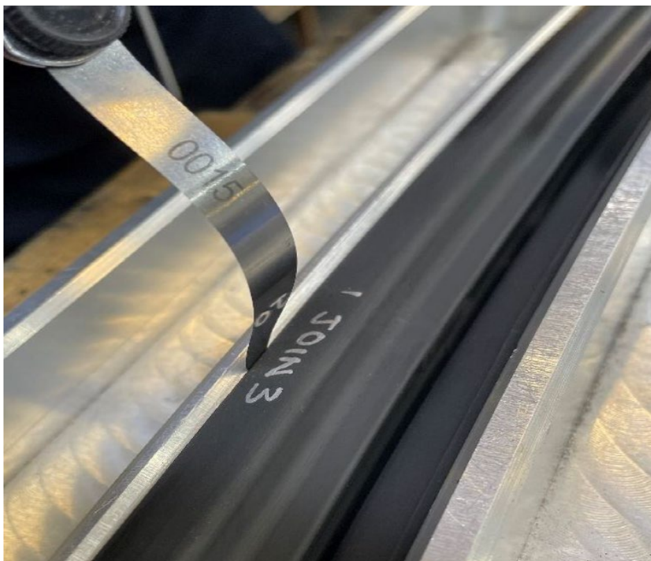
Image 4: Examination of join area with feeler gauge
